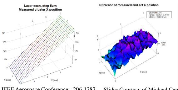
Standard deviation of position determined by fit is **0.32** μm
