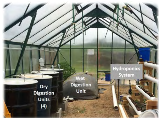
Fig. 2 Inside view of pilot-scale AD research at Ohio University where digestion units and a hydroponics system are managed together in a glasshouse enclosure to purposefully capture the wastes from one system to be used for the other. Water for both systems is obtained through a rainwater collection system (not pictured) installed on the glasshouse
