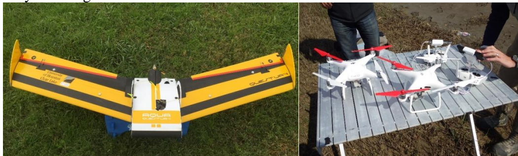
Figure 4. (Left) QUESTUAV AQUA 7ft fixed-wing Unmanned Aerial Vehicle and (Right) DJI Phantom 4 Pro Quadcopter with 20 megapixel camera.
