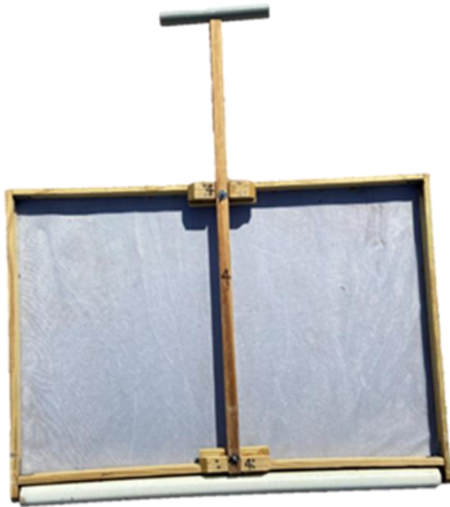
Figure 4. 1m 2 constructed pushnet (mesh size: 0.794 mm or 1/32 in).
