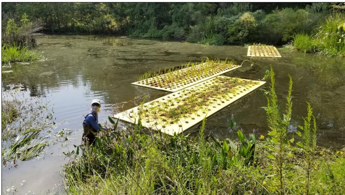
Figure 14. Kaylei Chau deploying the DIY FTWs into the holding area after planting. One mat contains a monoculture of Swamp Lily, one with Virginia Iris, and one with Swamp Smartweed. Not pictured is the control mat located at SS-F.
