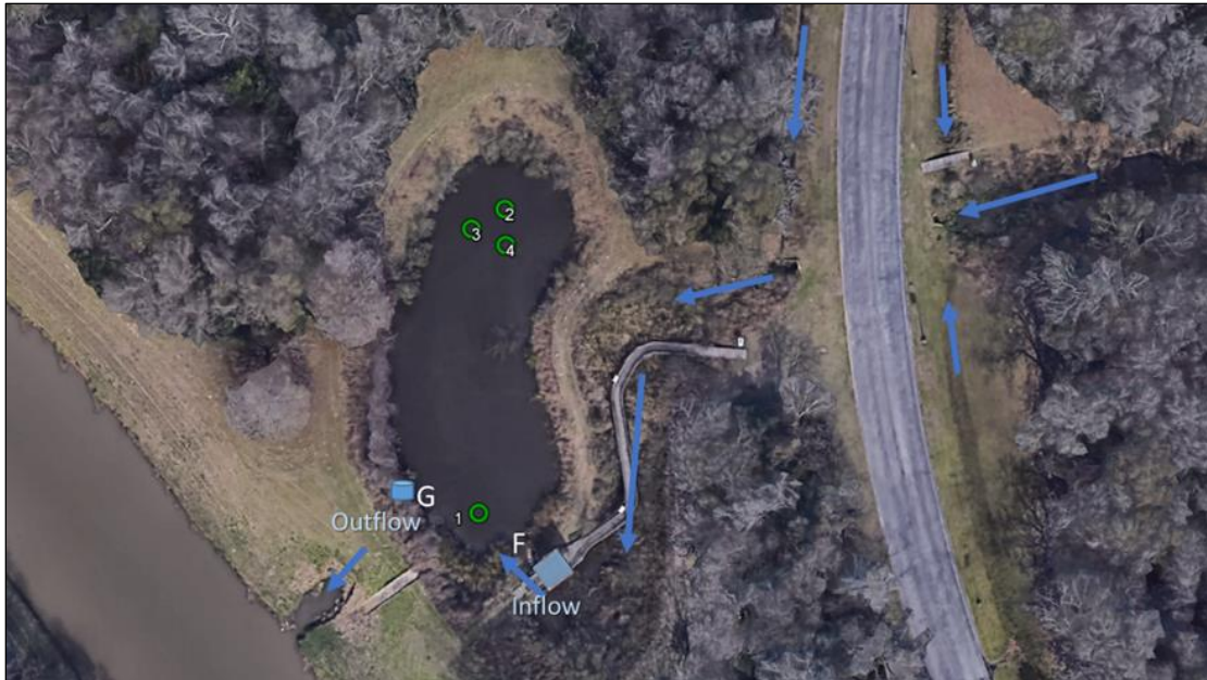
Figure 13. Monitoring Station 2 (Alligator Pond) with corresponding Sampling Stations F and G. The green circles numbered 1-4 represent the four mat types. The mat being tested for treatment potential would be placed directly in between the inflow and outflow while the mats that were not being tested during an event would be out of the main flow path in a holding area.
