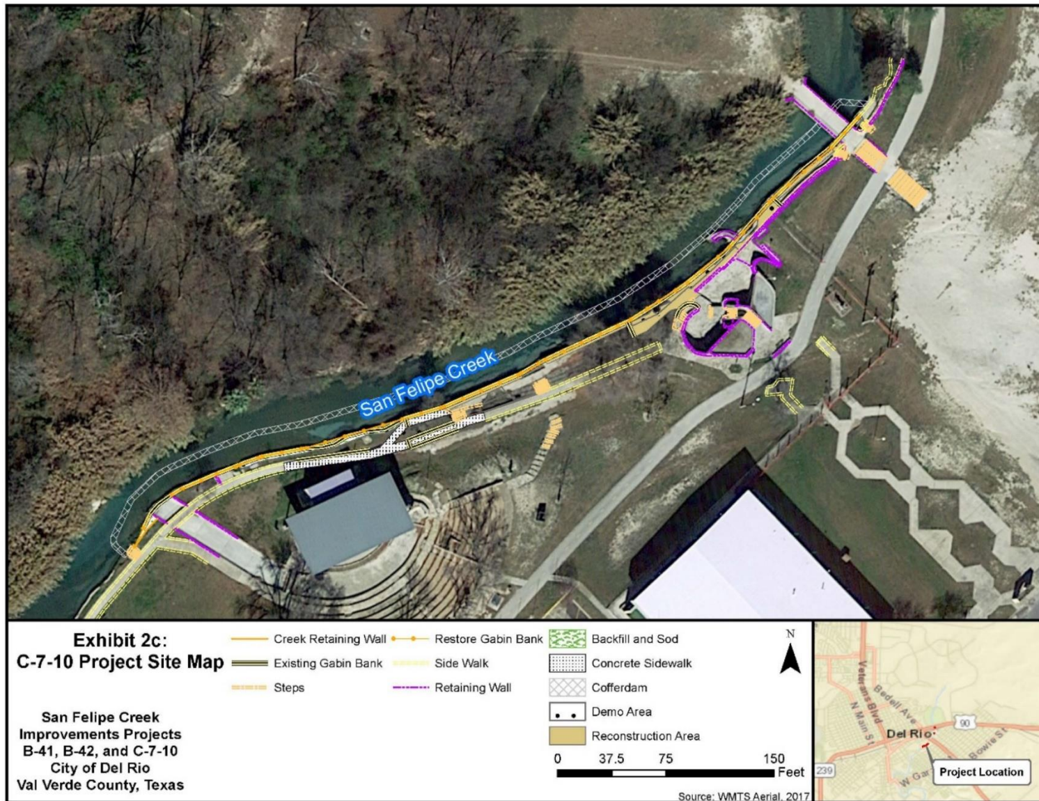
Figure 3 Approximate location of cofferdam installation area based on construction plans provided to the City of Del Rio, Texas.
