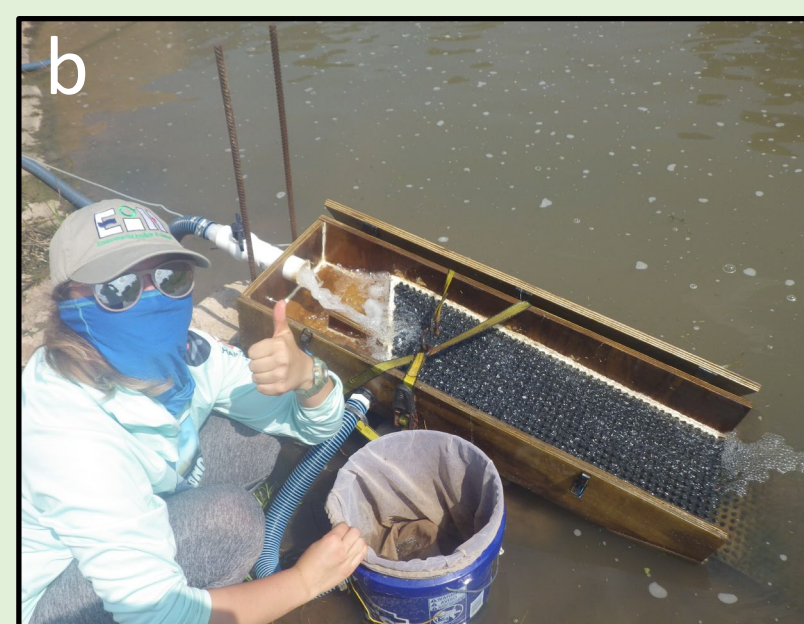
Figure 3. a: Gravity-fed eel ramp deployed at site 113. b: Example of target flow over ½” sheet drain and collection bucket at site 44.
