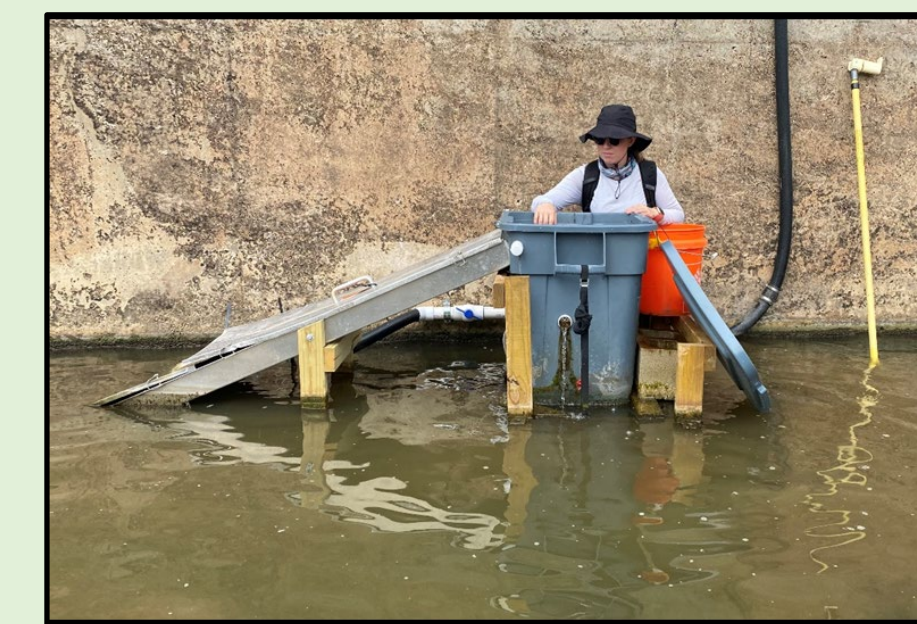
Figure 4. LCRA eel ramp deployed at site 120. Designs have varied slightly during study period.
