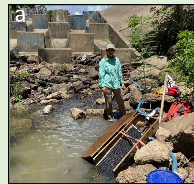
Figure 3. a: Gravity-fed eel ramp deployed at site 113. b: Example of target flow over ½” sheet drain and collection bucket at site 44.
