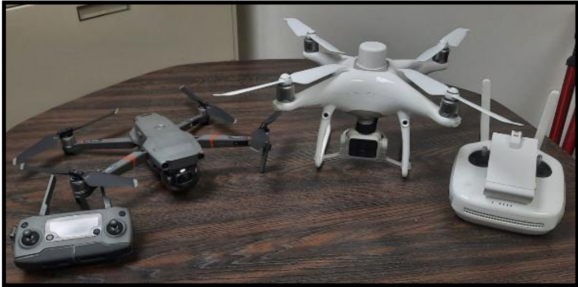
Figure 6: Drone or Small unmanned aerial system (sUAS) platforms used for aerial surveys: DJI Mavic 2 Enterprise Dual (left) and DJI P4 Multispectral (right).
