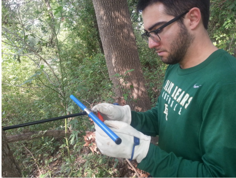
Figure 12. Crewmember collects tree core samples in the field.
