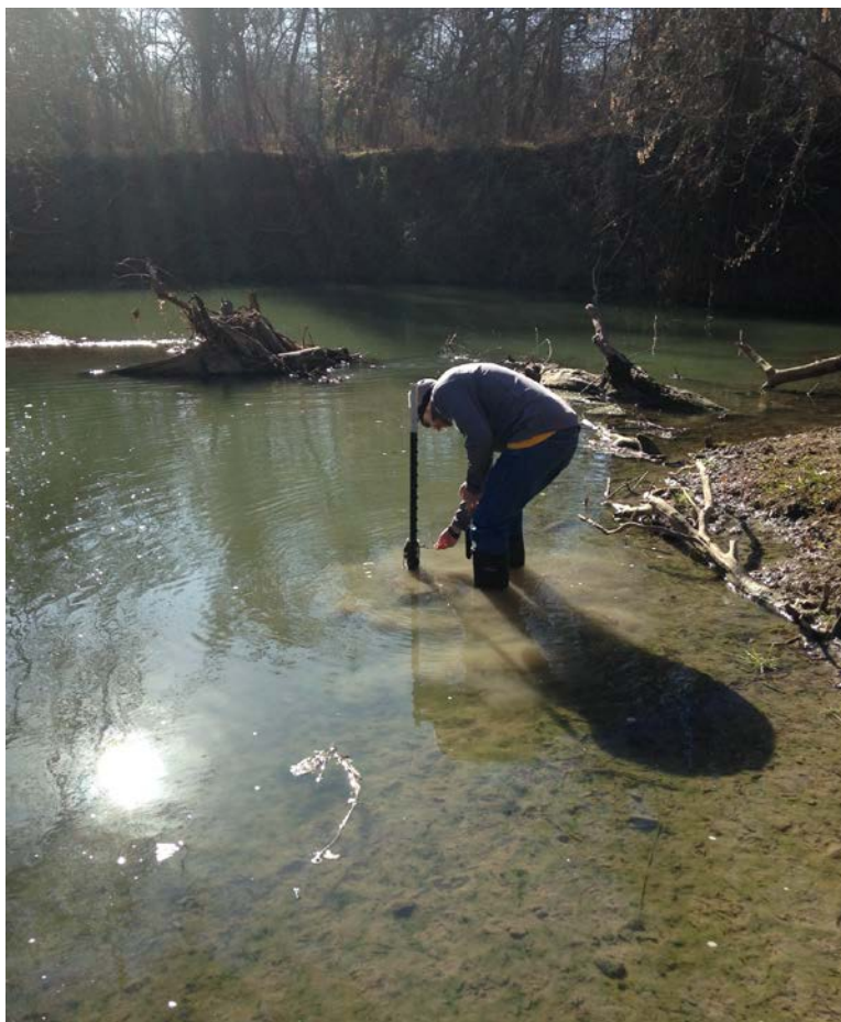
Figure 11. Crewmember installs a stream level logger.
