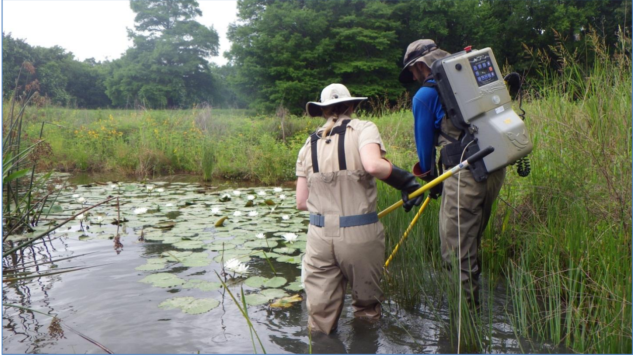
Figure 24. EIH staff sampling for nekton using a backpack electroshocker in the Secondary Wetland complex at the UHCL created wetlands.
