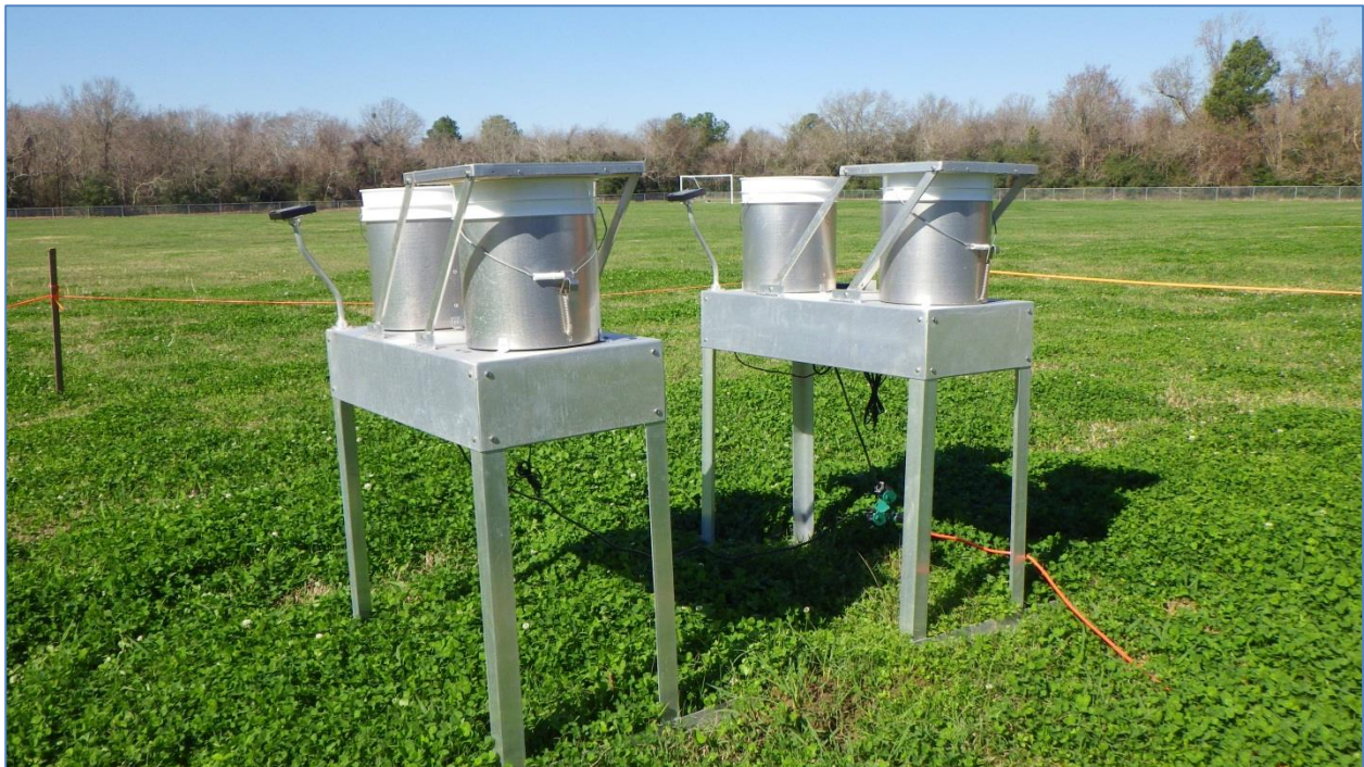
Figure 17. Dry deposition and precipitation samplers deployed in the field near the N.O.A. building on the UHCL campus.
