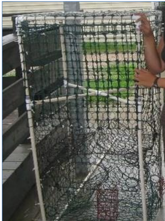
Figure 2. Modified crab trap, designed by Emma Clarkson. This terrapin trap consists of two crab pots wired together, with both roofs removed ensuring the terrapin's ability to find the chimney. The top 3 feet of the trap is open chimney surrounded by plastic fencing, preventing terrapin death by drowning.
