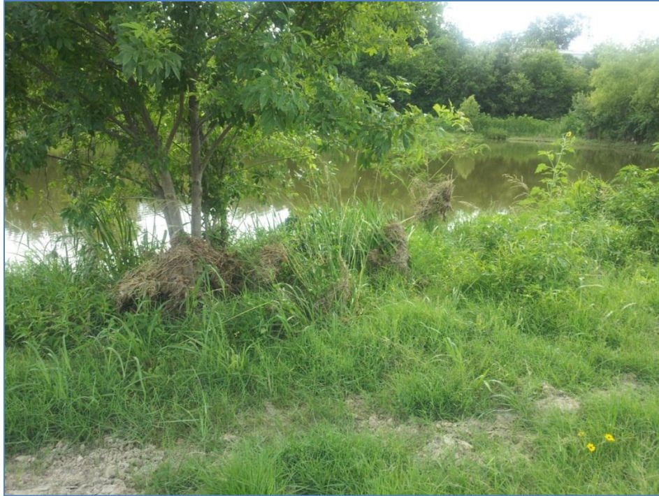
Figure 12. Debris line observed on June 31, 2012, at the edge of pond 1 marking recent maximum water levels during last flood event.
