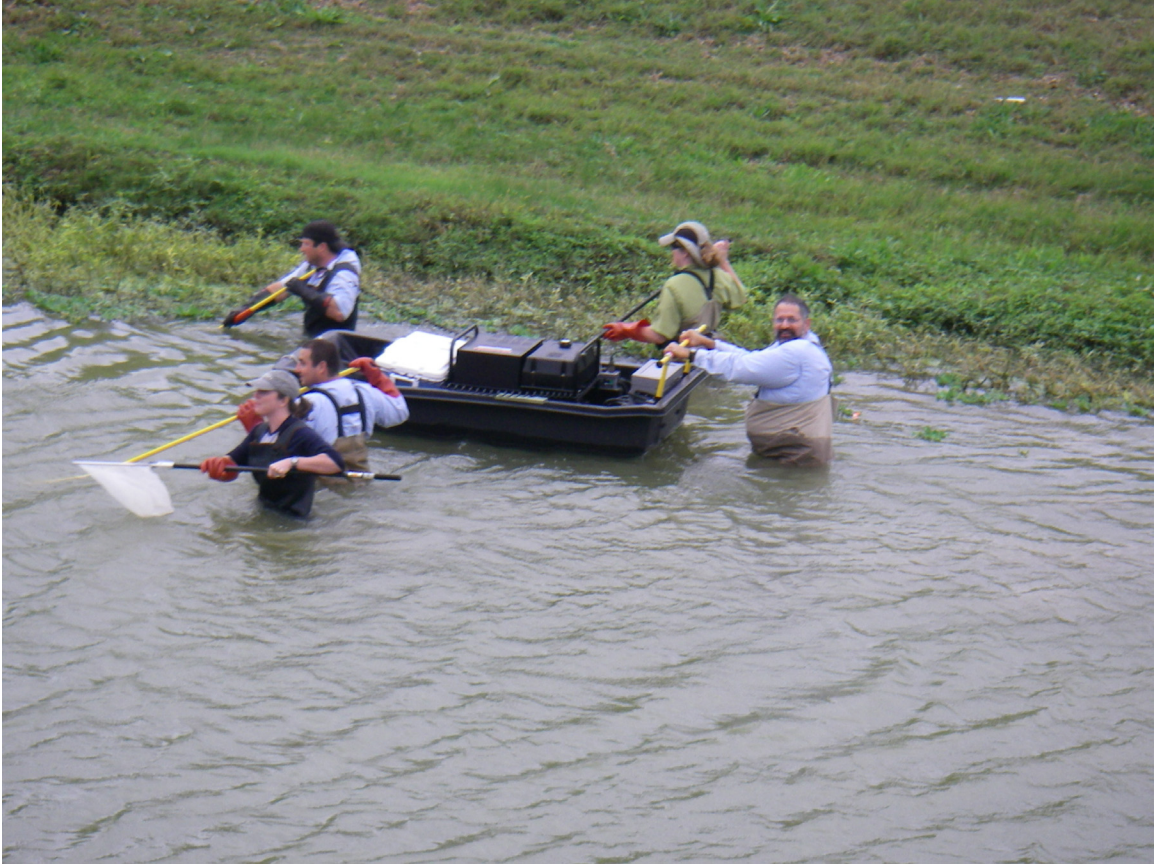
Figure 2. Electroshocking tote barge used to collect fish specimens.
