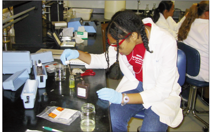
A GRADE camper uses a titration test kit to determine the chloride content of her water sample.
