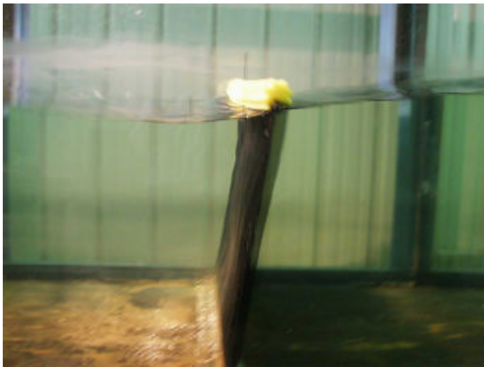
Figure 3. A photo showing the test of a flexible porous wave barrier in the wavetank.
