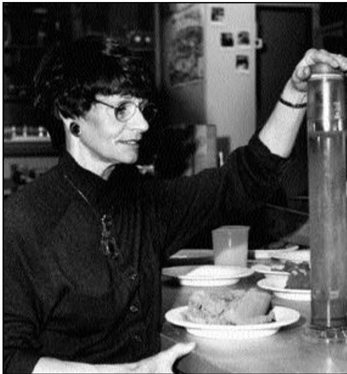
Prof. Theron Garcia is shown using a settling tube to determine the total suspended solid distribution in Galveston Bay samples.
