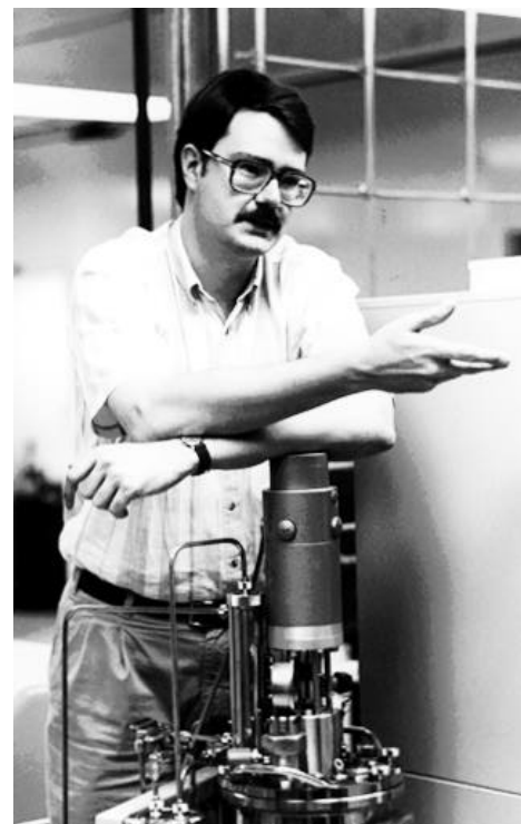
Dr. Richard Willson stands at an industrial fermenter utilized in experiments requiring large quantities of recombinant organisms.
