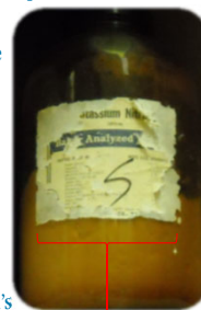
This container still contains chemical and the manufacture label on this container is not legible. It is required BY LAW to be re-labeled.
